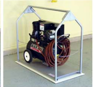
Air Compressors (Works in Attic)
