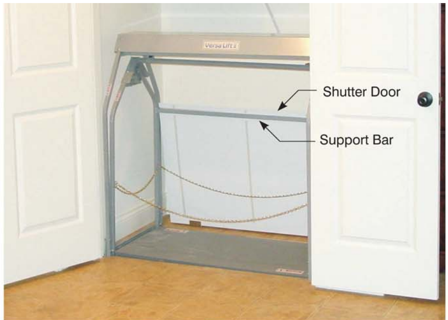
Fig. 1: When the lift platform is up, the shutter door rests on a support bar.
